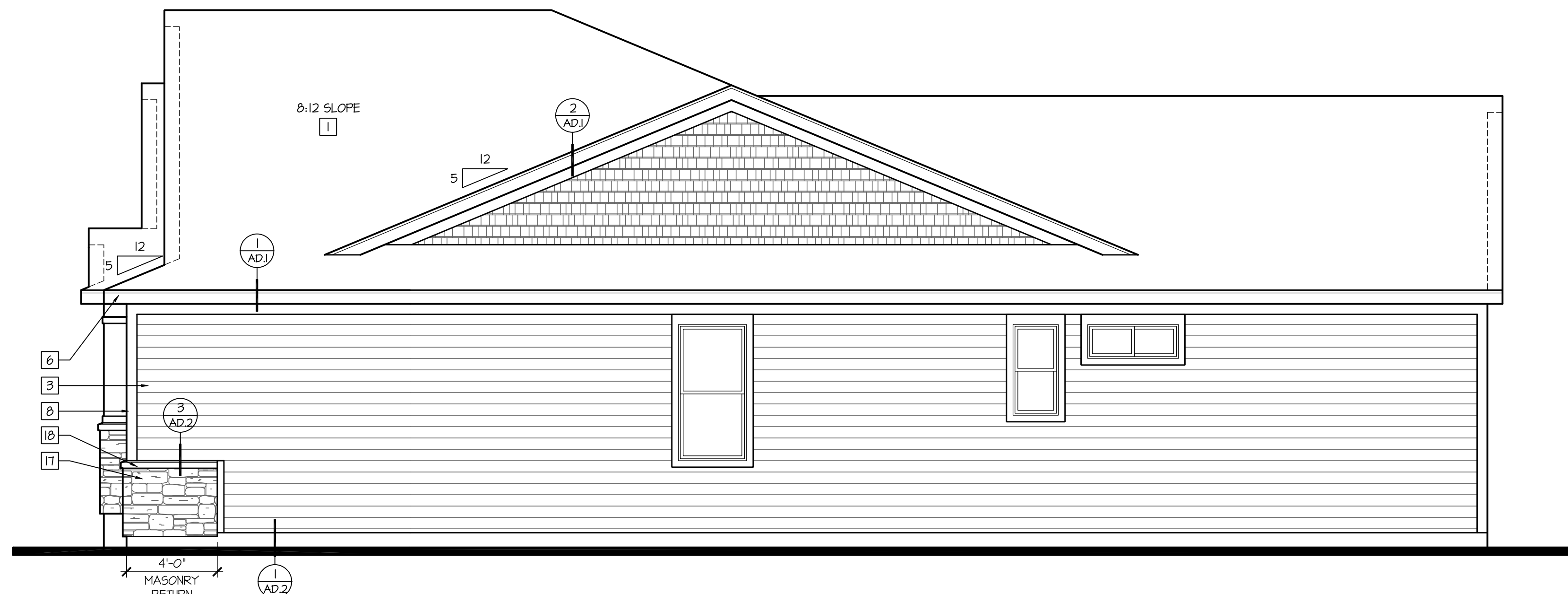
Right Elevation at End Wall Condition
